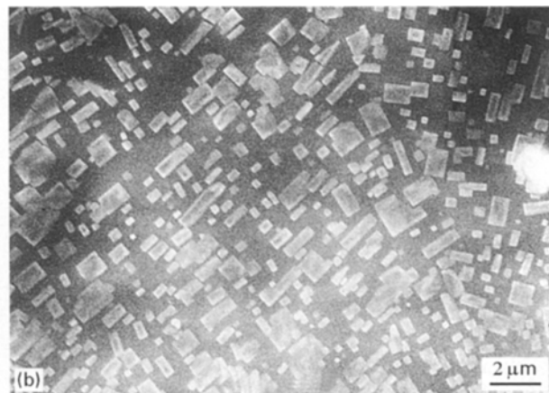
Figure 2 Scanning electron micrographs of calcite precipitated in solutions of (a) deionized water, (b) 1 wt % colloidal starch.
